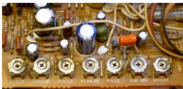
The pots have common-sense labels, from L to R: H-HOLD is the adjustment for the Horizontal Hold (H synchronization)
