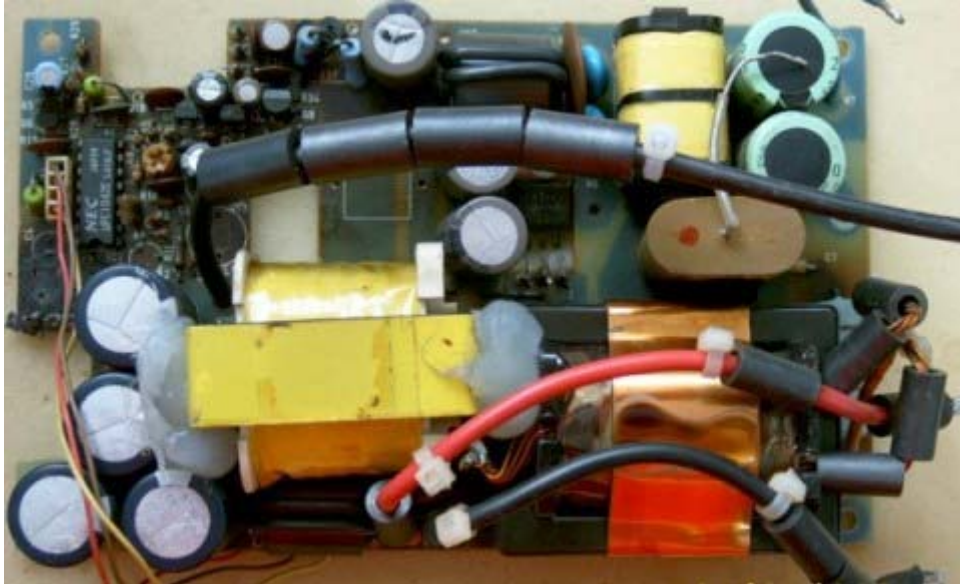
The REG PCB with most of the original parts on it; A few of the overheated parts near R32 area were already removed.
