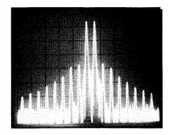
Fig 3—Spectral display of the IC-781 during two-tone intermodulation distortion (IMD) testing. Third-order products are approximately 37 dB below PEP output, and fifth-order products are approximately 39 dB down. Vertical divisions are each 10 dB; horizontal divisions are each 2 kHz. The transceiver was being operated at 150 W PEP output on 14.2 MHz.
