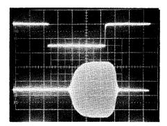
Fig 4—CW-keying waveforms for the ICOM IC-781 in the full-break-in mode. The lower trace is the RF envelope; the upper trace is the actual key closure. Each horizontal division is 5 ms. The IC-781's CW keying is extremely good.
