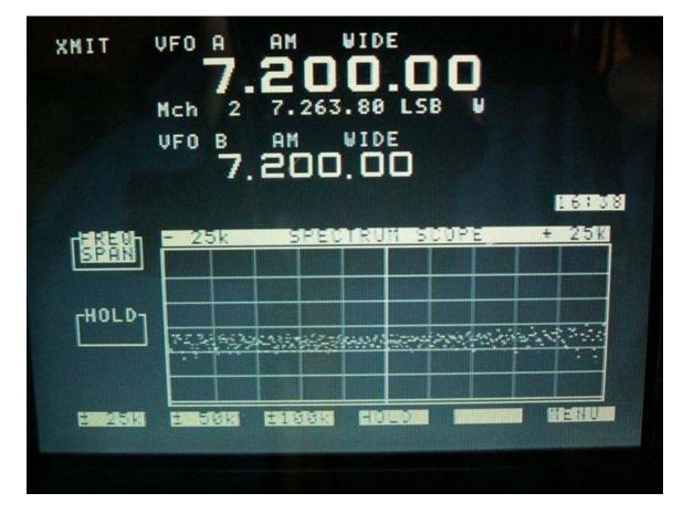
Original IC-781 Spectrum Scope display with no roofing filter:
