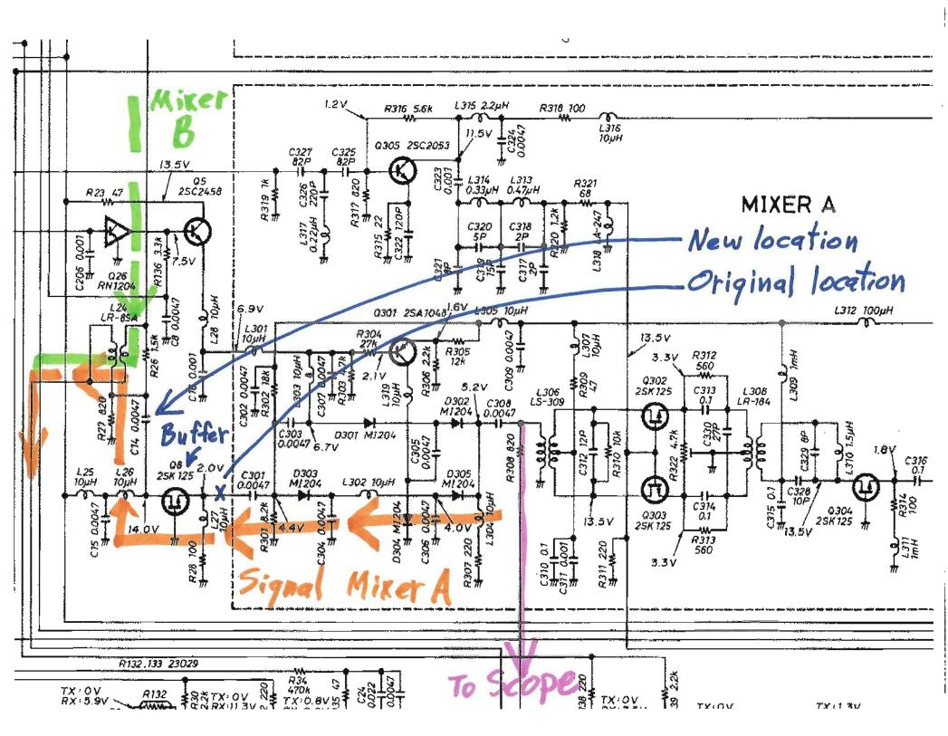
Alternative IC-781 INRAD roofing filter installation
