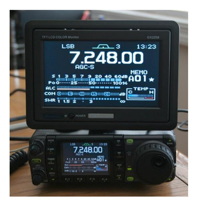
When I first looked at the 7000, I was a little shocked at the size of the screen. It measures only 2.5 inches diagonal which is noticeably smaller than the IC-706's antique LCD display.
