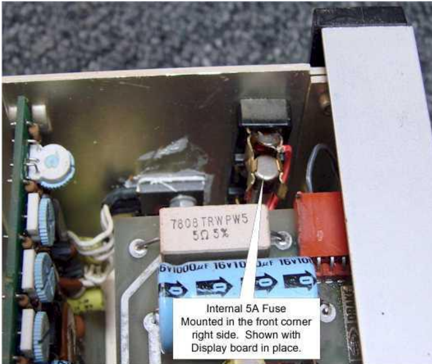
Front & Side views of 5A fuse location
