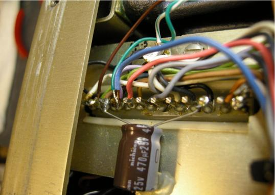
Illustration 3: Source of power for the PIN attenuator
