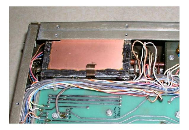
Picture 13: Shield for the lowpassmodule – lower side
