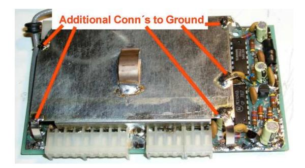
Picture 11: Shielding used as additional ground-layer
