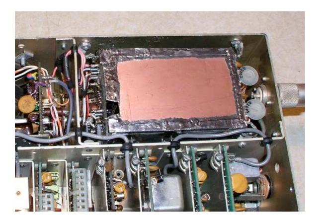
Picture 12: Shield for the lowpassmodule – upper side
