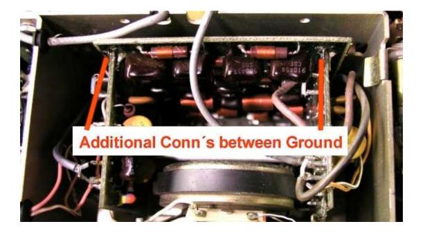
Picture 4: Additional groundconnections in the highpassmodule
