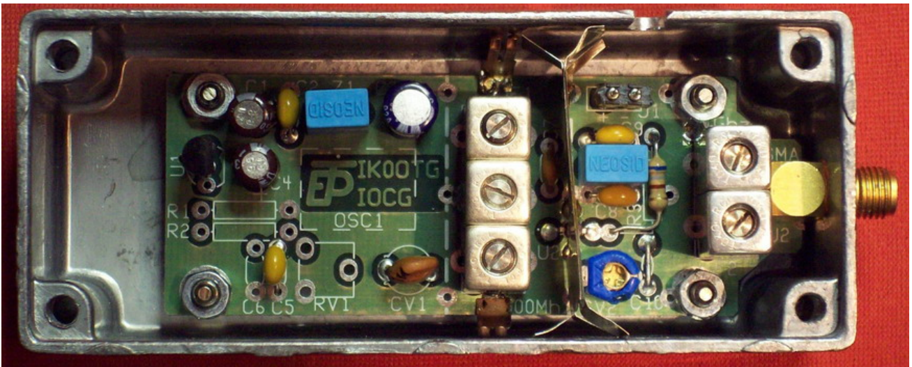
IOCG 1 GHz Clock Generator PCB assembly is fitted inside box
