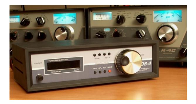
The DDS-4 is a complete Digital Tuning System, a VFO, with full control of DRAKE R4 receivers and T4 transmitter. It use a modern DDS AD9951 frequency generator and a PIC microcontroller.
