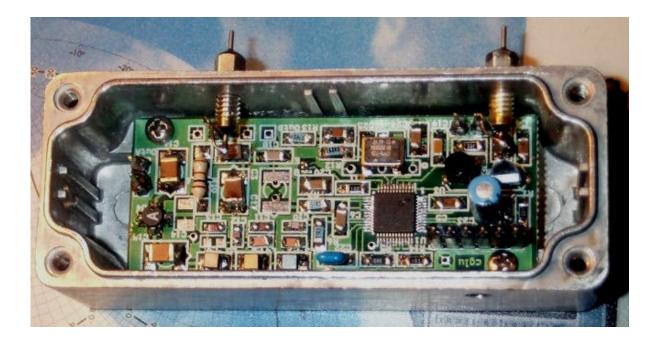
THE PIC CONTROL PANEL ASSEMBLED (the picture not display the DDS-4 application software)
